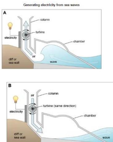
The diagrams show a structure that is used to generate electricity from wave power. Summarise the information by selecting and reporting the main features, and make comparisons where relevant.
